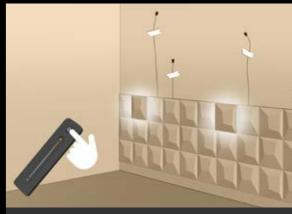
4. Connect the LED accessories to the power supply and make sure the panels light up when each one is installed.
